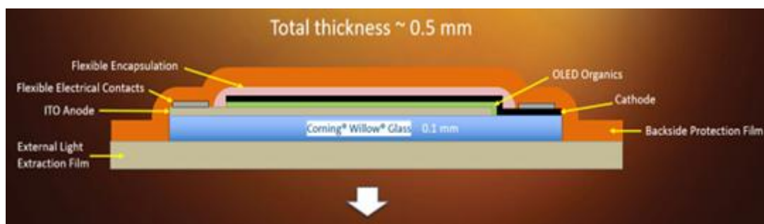
Figure 4.2: Construction of an OLED, Source: [14]
